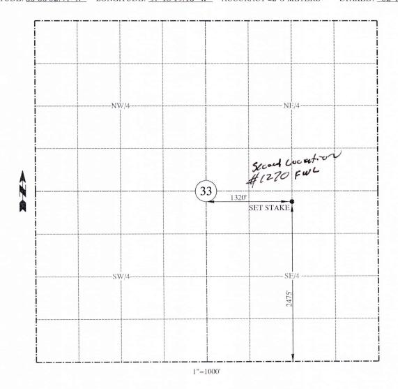
DISTANCES SHOWN ARE BASED ON THE QUARTER SECTION BEING 2640 FEET. ACTUAL SECTION LINE DISTANCES HAVE NOT BEEN MEASURED. THIS PLAT DOES NOT REPRESENT A BOUNDARY SURVEY.
